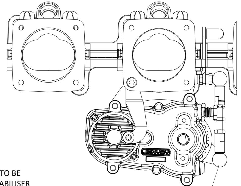
BRACKET M5 X 20 BOLTS SECURE ONTO BOTTOM FLANGE OF THROTTLE BODIES
