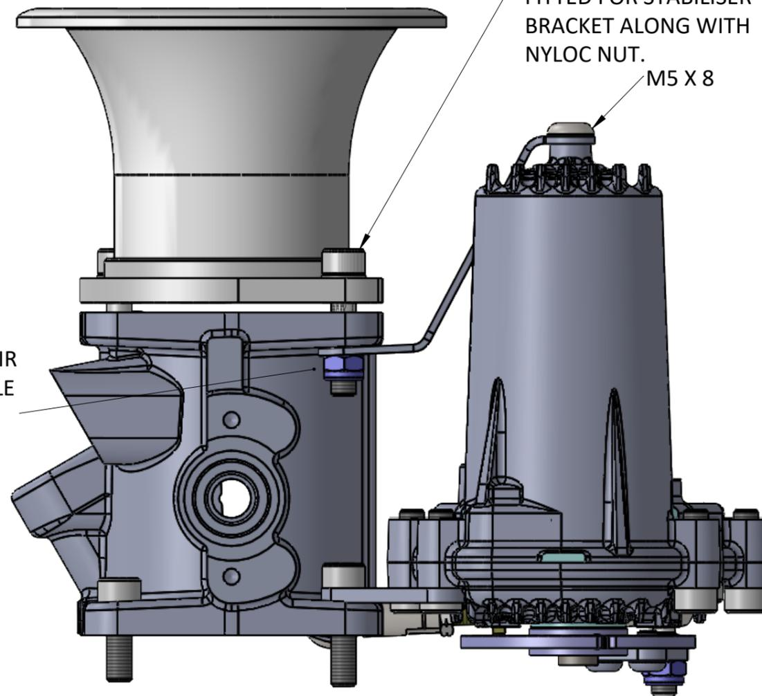
M5 X 25 BOLT TO BE FITTED FOR STABILISER BRACKET ALONG WITH NYLOC NUT.
